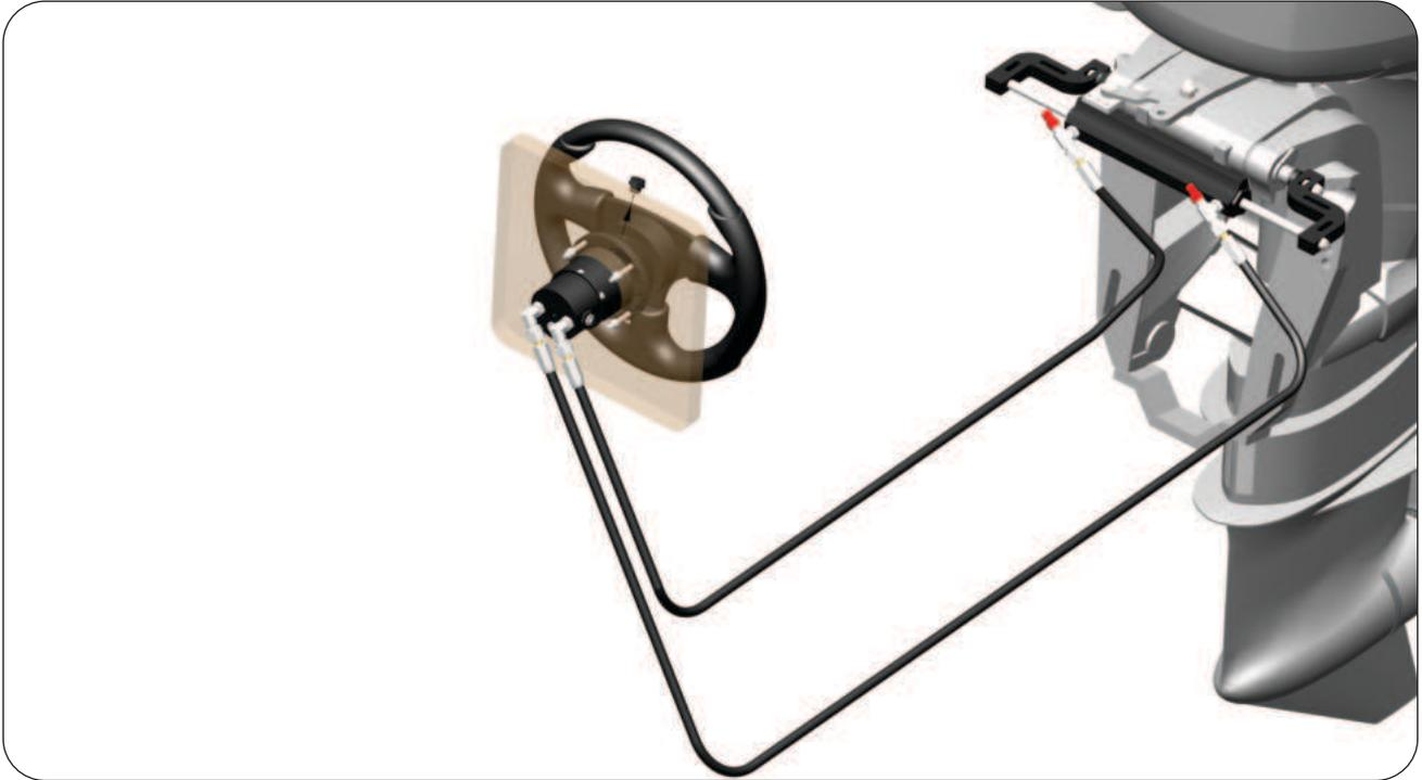
**STEP 10 :** Insert the threaded Port of pipe into the Oil Filling Port of Helm. Turn the bottle upside down and carefully remove the other side of cap to ease the Oil passage towards the Helm. Fill the Helm until no air bubbles are visible in the pipe.
