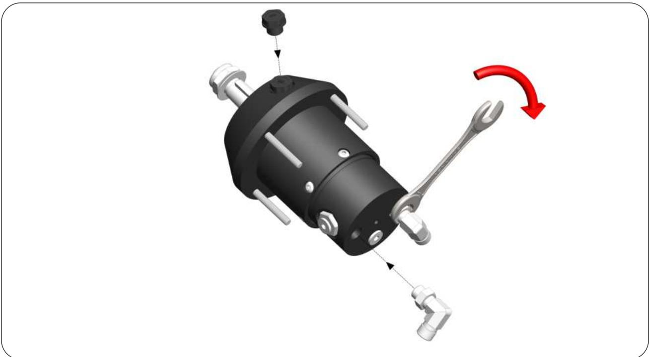
**STEP 6 :** Insert the Helm from the front of the dashboard with the Vented Plug (9) turned upwards matching the 4 Flange Studs (5) moving inside the 4 holes on the dashboard.
