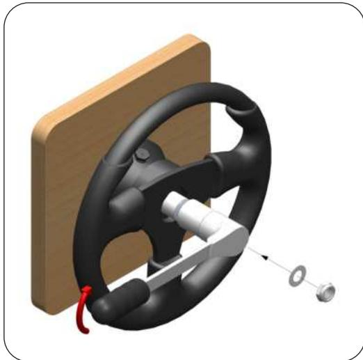
**STEP 3 :** Fit the Steering Wheel on the Shaft by inserting the Specific Key (1) in its compartment. Insert the Washer (2) and use a 20mm hexagonal Wrench to tighten the Self-Locking Nut (3) with a 40 Nm (29.5 lb ft) torque.
