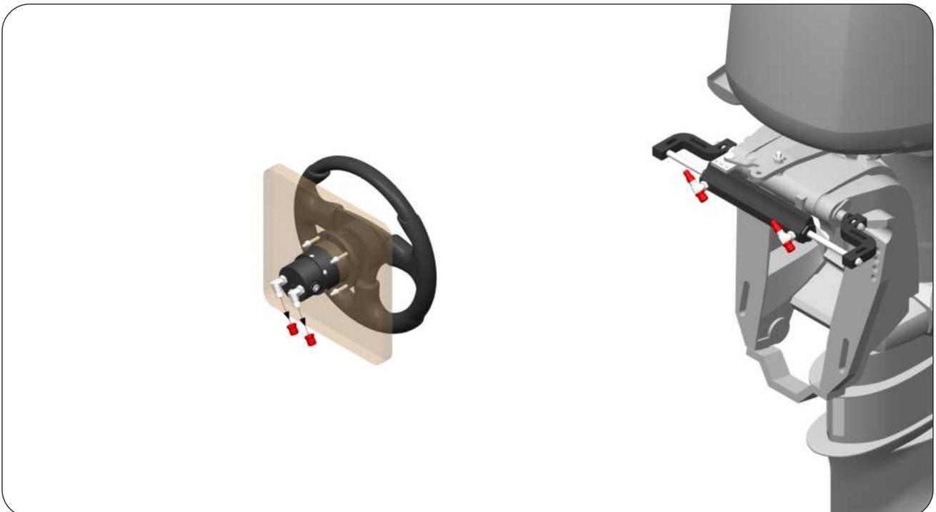
**STEP 3:** Insert the Hose Fittings into both the Elbows of Helm. Tighten the Hex Nut on the Hose Fitting by using 19 mm Wrench with a torque of 15 Nm (52 lb ft).
