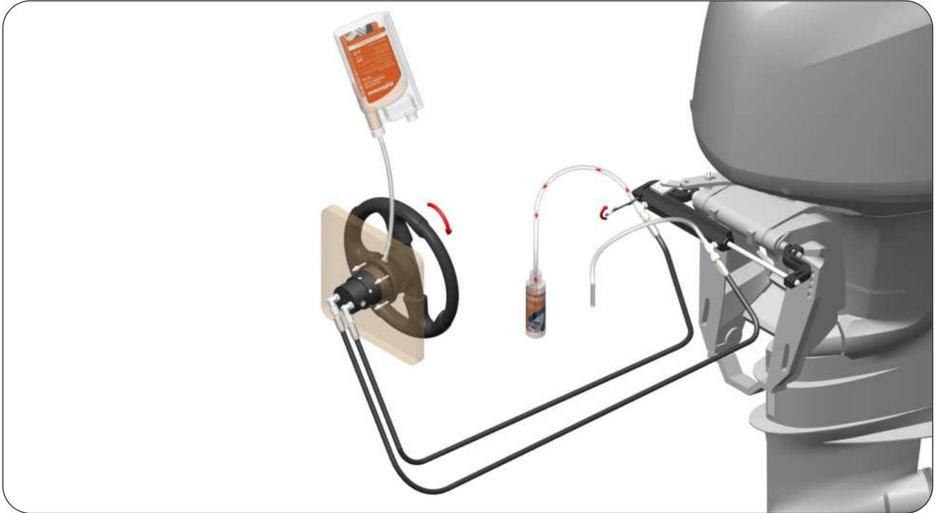
**STEP 16 :** Continue to turn the Steering Wheel towards Port Side. When the Oil comes out from air bleeder without air bubbles then carefully close the air bleeder. Do not overtighten the air bleeder. Continue to turn the Steering Wheel in the same direction to fill the Cylinder chamber. During this phase the Cylinder body will move to the opposite direction up to the end stroke.
