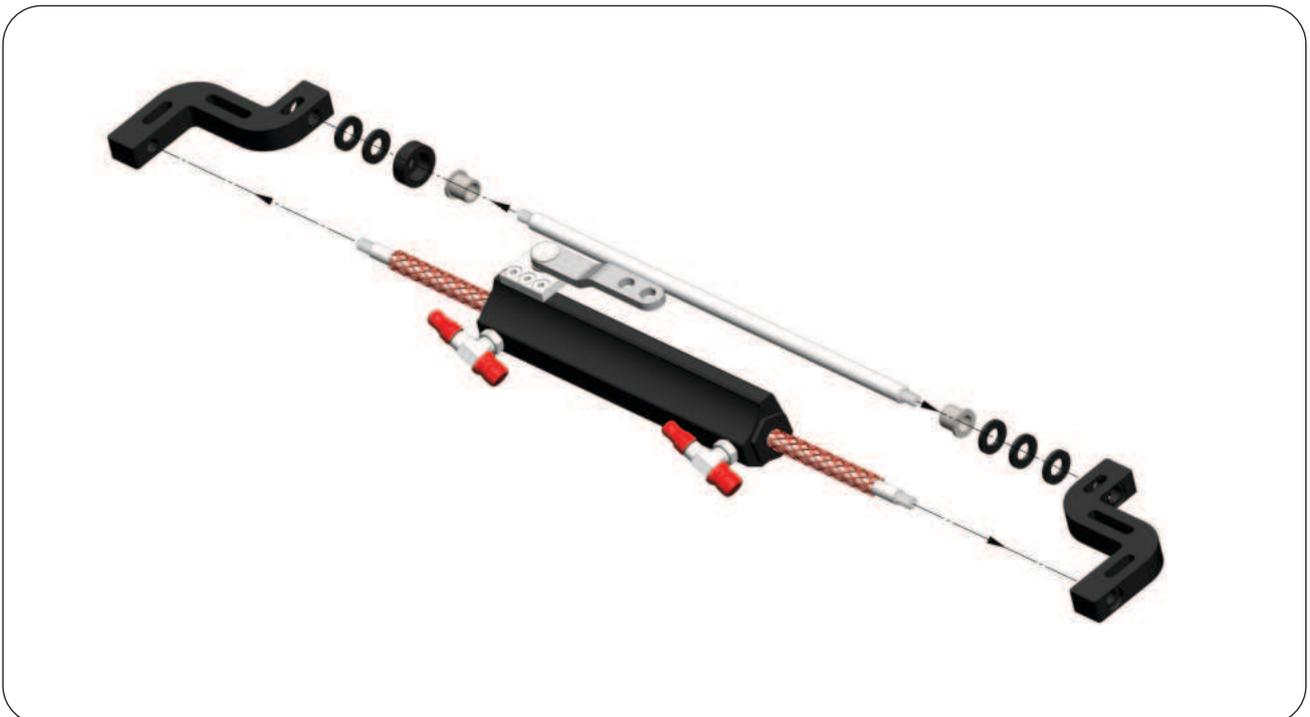
**STEP 3:** Apply Marine Grade Grease on the Center Shaft (4) and insert the Center Shaft into the Tilt Tube of Engine.
