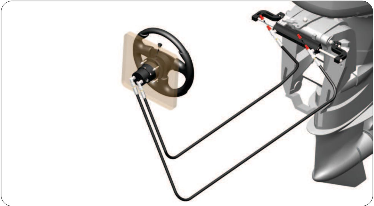
**STEP 18 :** After tightening the Oil Filling Plug, some amount of Oil will come out around the plug for some period of time when the Wheel is turned lock to lock. This Oil seepage will be over when the system is stabilized and no air is trapped inside the system.
