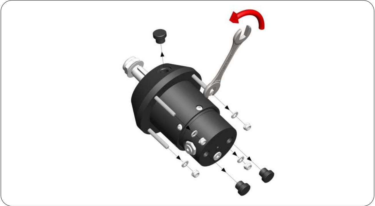
**STEP 5 :** Insert and tighten by hand the Elbow Fittings (8) until they are fully seated, then tighten with a wrench. Turning again from 1.5 to 2.5 turns, for their best orientation for the Hose connection. However do not exceed a maximum torque of 17.6 Nm (13 lb ft). Also insert the Vented Plug (9) into Oil Filling Port.
